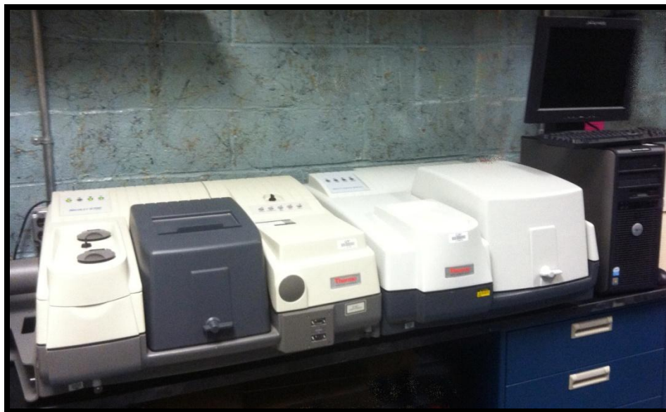
Figure 18. A Thermo NXR FT-Raman Instrument (InGaAs detector), which can be used for both Fourier transform infrared spectroscopy (left) and Raman (right) spectroscopy [John Jay College of Criminal Justice, CUNY].
