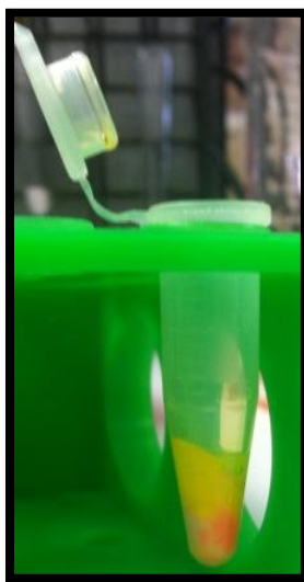
Figure 83. Resultant extraction of Dolemite tattoo ink. Note the presence of three distinct color profiles- white (bottom), orange and yellow (top).
