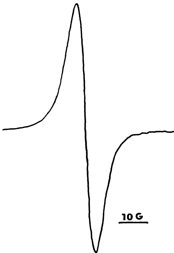
Figure 42. Room temperature ESR spectrum of the insoluble part of poly(1,4-diphenyl-1,3-butadiyne) in solid state.
