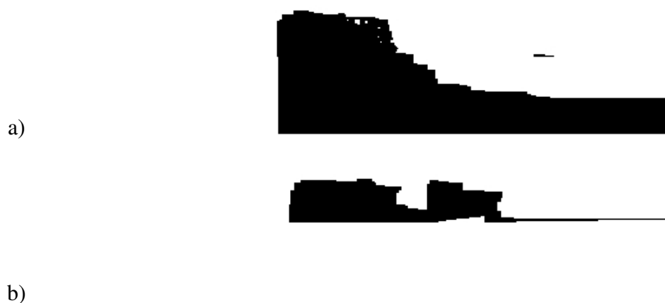
Figure 5.1: The hard segmentation of the noisy spectrogram with a) 5 dB SNR, and b) 0 dB SNR.
