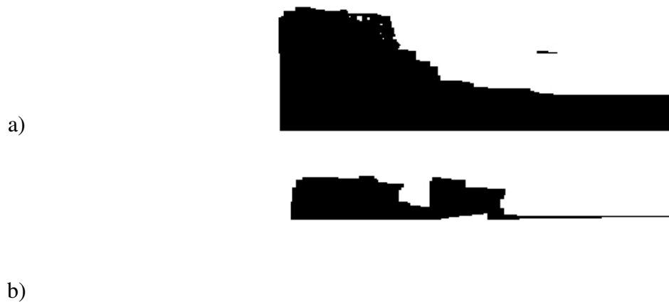
Figure 3.8: The hard segmentation of the noisy spectrogram with a) 5 dB SNR, and b) 0 dB SNR.
