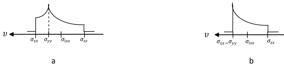
Figure 2.5: Chemical-shift powder pattern for a). Asymmetric anisotropy and b). Axially symmetric anisotropy
