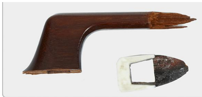
Figure 1.4: A broken violin bow's head with a separated head-plate, (copyright Tarisio archives)
