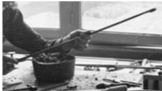
Figure 4.4: At the Mirecourt School, cambering a bow over ambers (copyright Benoît Rolland)
