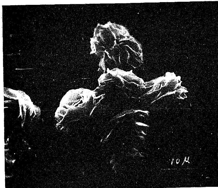
Fig 2.2 (c) Scanning electron micrograph of hedrites of 99%-trans-polybutadiene grown from 2% amyl acetate solution at 30°C by the direct cooling procedure.
