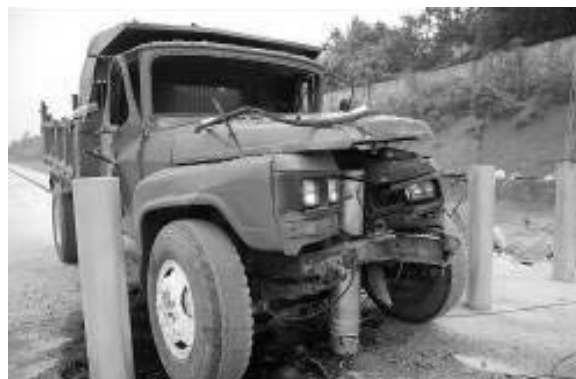
(d) Truck and bollards after the collision
