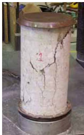
Figure 3.9 Concrete Cylinder Compression Test under Quasi-static Load.
