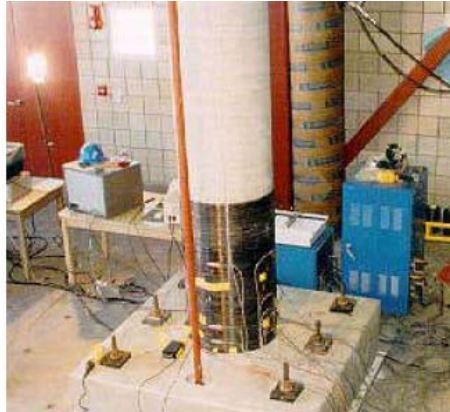
Figure 6.1 Testing of the FRP Wrapped Bridge Piers
