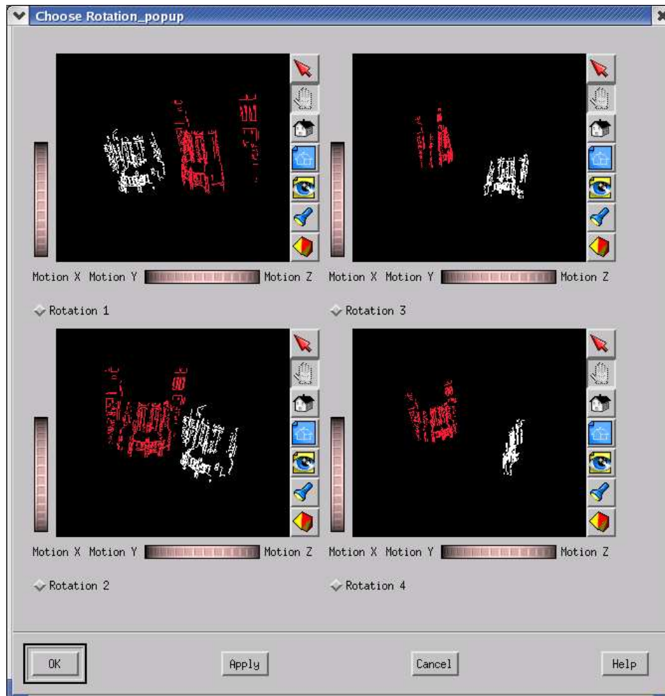
Figure 5.6: A set of possible orientations between the two coordinate systems is presented to the user to choose from. In this example, the rotation in the upper left corner corresponds to the correct result.
