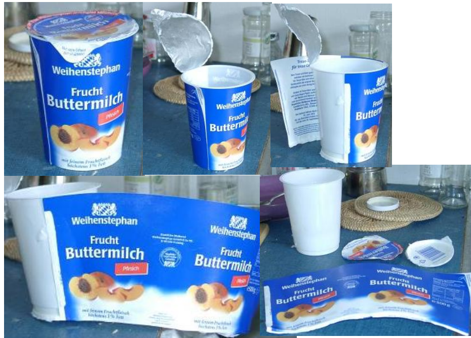
Figure 10: Easy detachment of different parts in a fruit buttermilk cup
