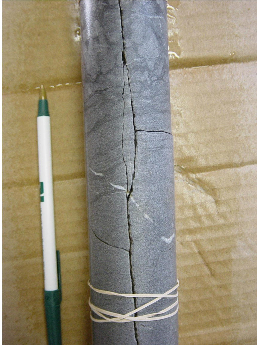
Figure 83. Beekmantown core. An extension fracture passing through a parasequence boundary. This parasequence is an upward coarsening storm parasequence, identified by the presence of a round-pebble conglomerate at the top of the parasequence. Beds become thinner at the top of the parasequence, indicating a change from a subtidal zone to an intertidal or supratidal zone. This fracture is classified as a non-strata bound fracture, since it was not constrained by either the bedding planes or the parasequence boundary (Needham, 2005).
