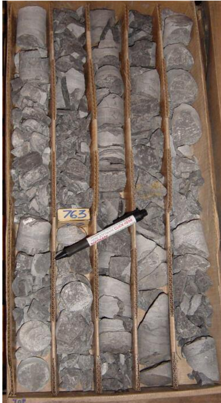
Figure 9. Carbonate rubble from core sample 74-NY-11. Depth interval 231 to 234 meters (757 to 767 feet). Despite the severe degree of deformation, some shear fractures can be seen in the core. These fractures intersect the core at an acute angle to the vertical axis of the core.
