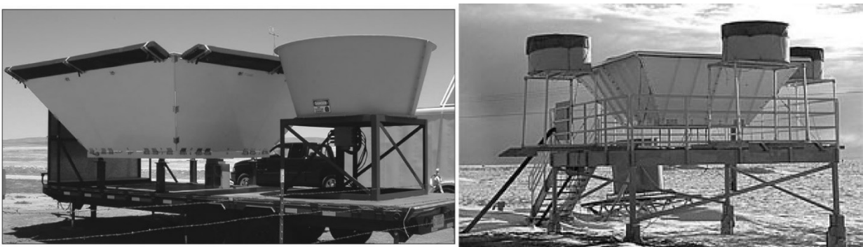
Figure 5, Image of a portable sodar wind profiler (left) and permanent radar wind profiler installation (right).[53, 54]
