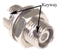
Figure 76, FC to FC bulkhead fiber optic adapter. Arrows indicate the keyway that allignes the angles tips of the FC connector.
