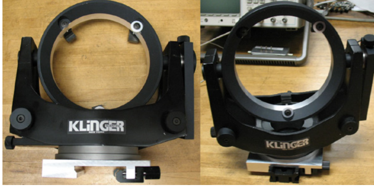
Figure 54, Picture of modified mirror mount secured to custom optical rail carriage (left) and same secured to an optical rail.
