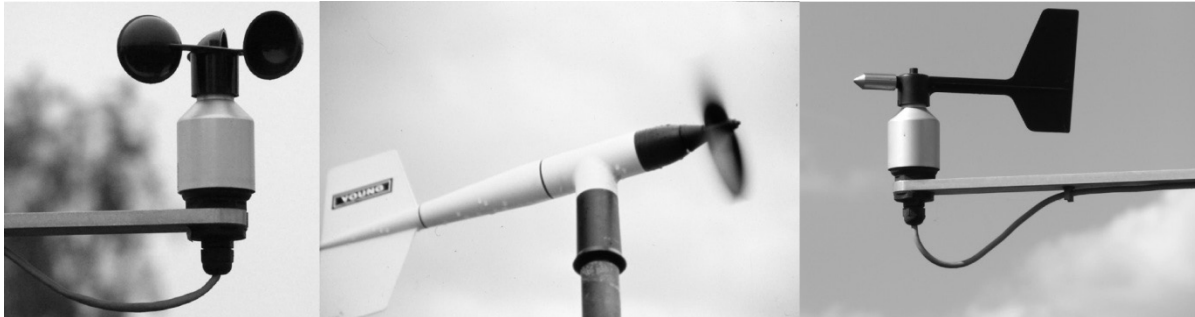
Figure 4, Image of cup anemometer (left), propeller anemometer (center), and wind vane (right).[50-52]
