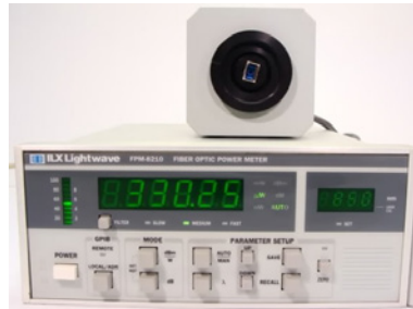
Figure 35, Fiber optic power meter by ILX, model FPM-8210 with integration sphere.
