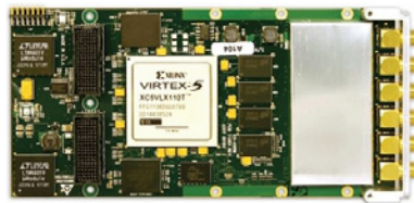
Figure 71, Data acquisition card X5-400M with two 14 bit ADC channels with a 400 MHz sampling rate.
