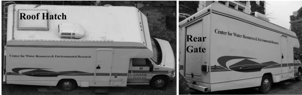
Figure 13, Research vehicle containing Lidar system. Images show location of roof hatch and rear rollup gate.
