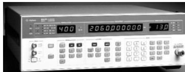
Figure 55, Hewlett Packard 8657B signal generator with 0.1 to 2000 MHz sinusoidal output frequency range.
