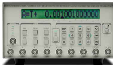
Figure 66, Digital delay generator from Stanford Research Systems used as a time keeper for system.
