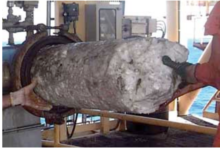
Figure 1.1: A gas hydrate plug taken from an offshore production line of Petrobras, Brazil.
