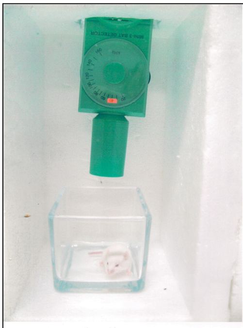
Figure 1: The ultrasonic vocalization apparatus. Animals are placed into a sound proof chamber with an ultrasonic frequency detector above. The number of vocalizations made by the animal is sent to a computer equipped with Ultravox software, which allows for quantitation of the number of vocalizations emitted by the animal.
