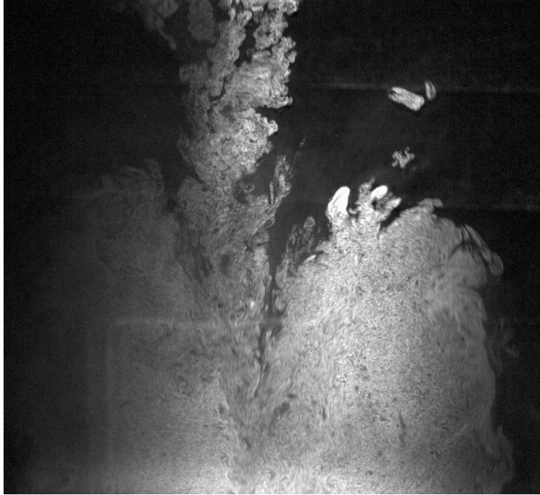
Figure 6-16: Flow visualization with laser sheet at y=9\text{cm} with panel at 83^\circ deployment
