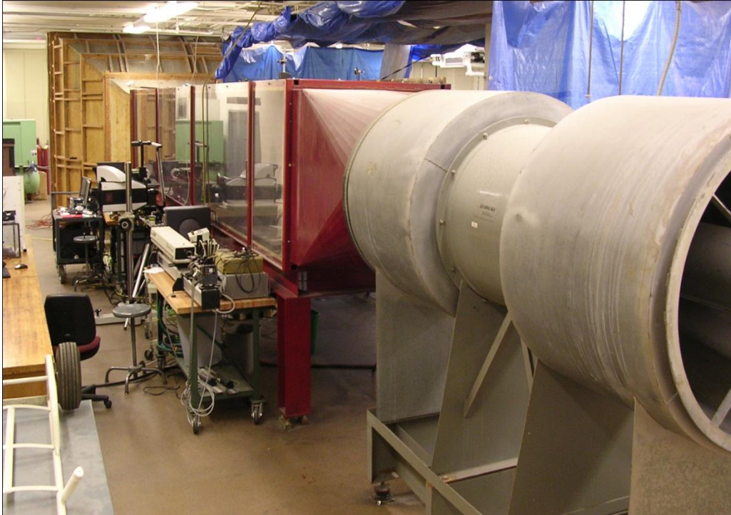
Figure 2-2: Photograph of the wind tunnel facility
