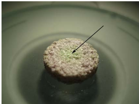
Figure 4.11. Macro-porous SiO 2 glassy sample impregnated by Cr 4+ :Ca 2 GeO 4 sol and subjected to heat-treatment (650°C, 20hr). Green spot in the middle is due to Cr 4+ :Ca 2 GeO 4
