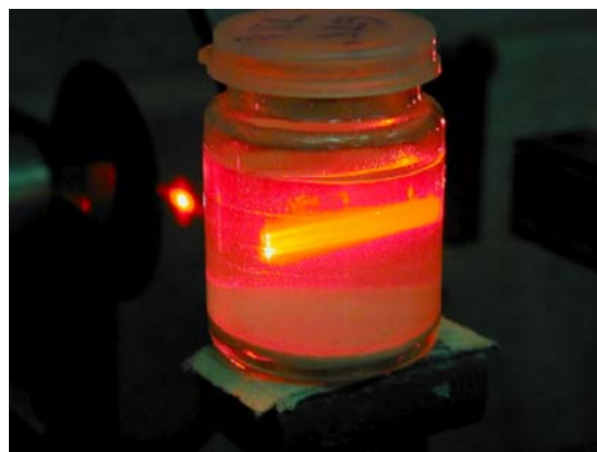
Fig.4.4. Light scattering of Sol-gel Cr:Ca 2 GeO 4 powder in methanol.
