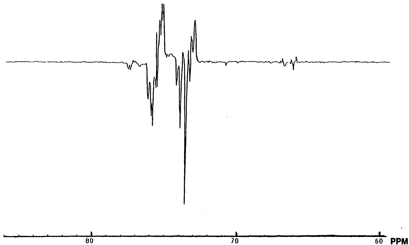
Figure 22. 50.3 MHz 13 C-NMR DEPT spectrum of PPO prepared with Al.DMBD initiator. CH (positive) and CH 2 (negative) region. Conditions: 30° pulse angle; 24°C; 3772 acquisitions; 10s relaxation delay.
