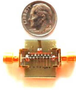
Figure 4.3 Fabricated 7-section LH NLTL phase shifter using FR4 substrate
