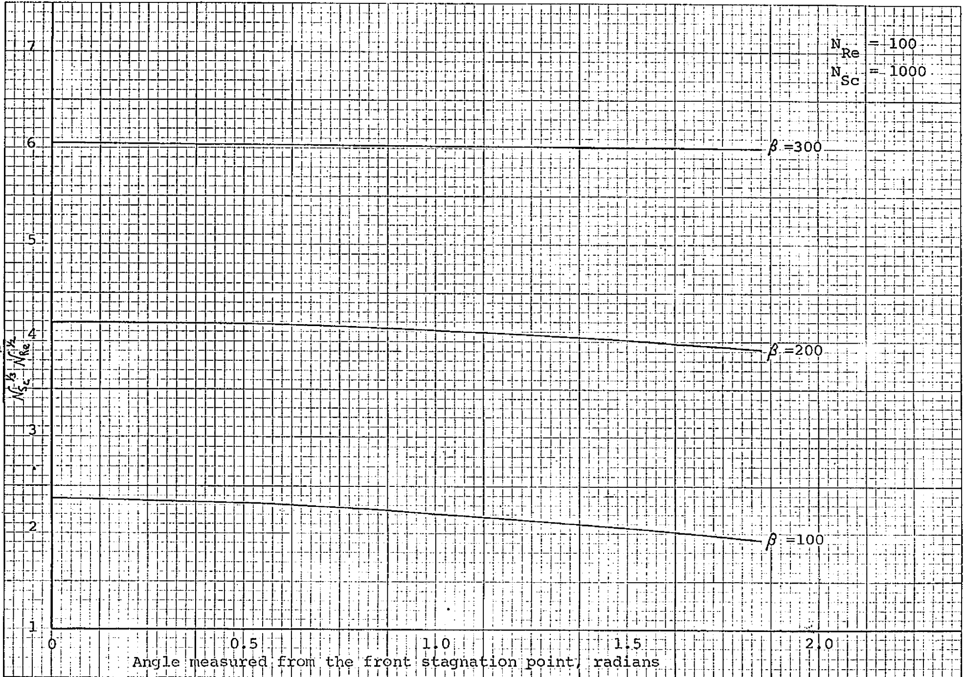
Fig. 4: Effect of high reaction rates and hydrodynamic behavior at N_{Re} \gg 1 on local mass transfer around single solid spheres
