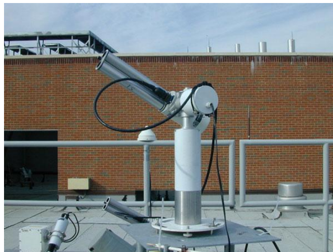
Fig. 19: A sunphotometer used to obtain aerosol particle size distribution.
