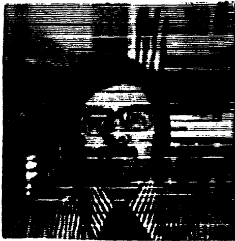
(a) Noisy picture; 3 \times 10^{-4} error rate; 1024 bits/line; 170 lines.
