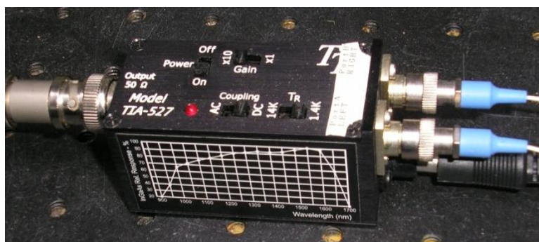
Figure 2-15 The InGaAs optical balanced detector used to retrieve backscattered signals.
