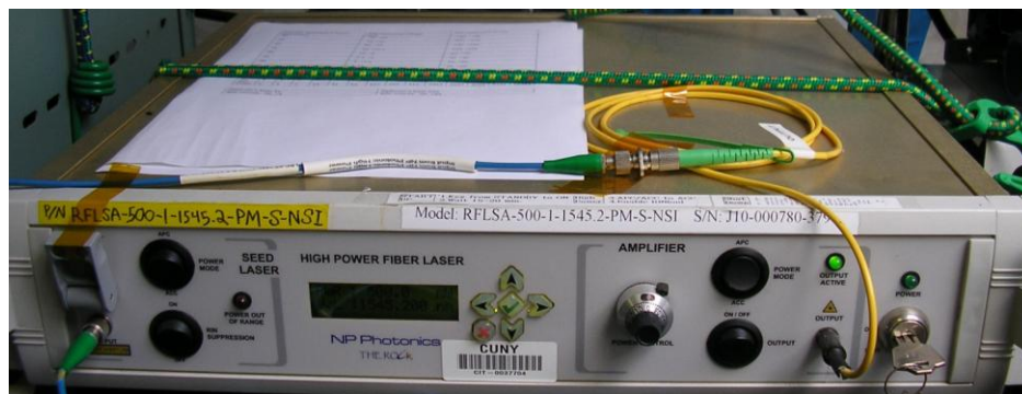
Figure 2-2 The fiber optics Laser source that has two laser outputs; one output is a low power that is used as a seed laser, the other output is a high power.
