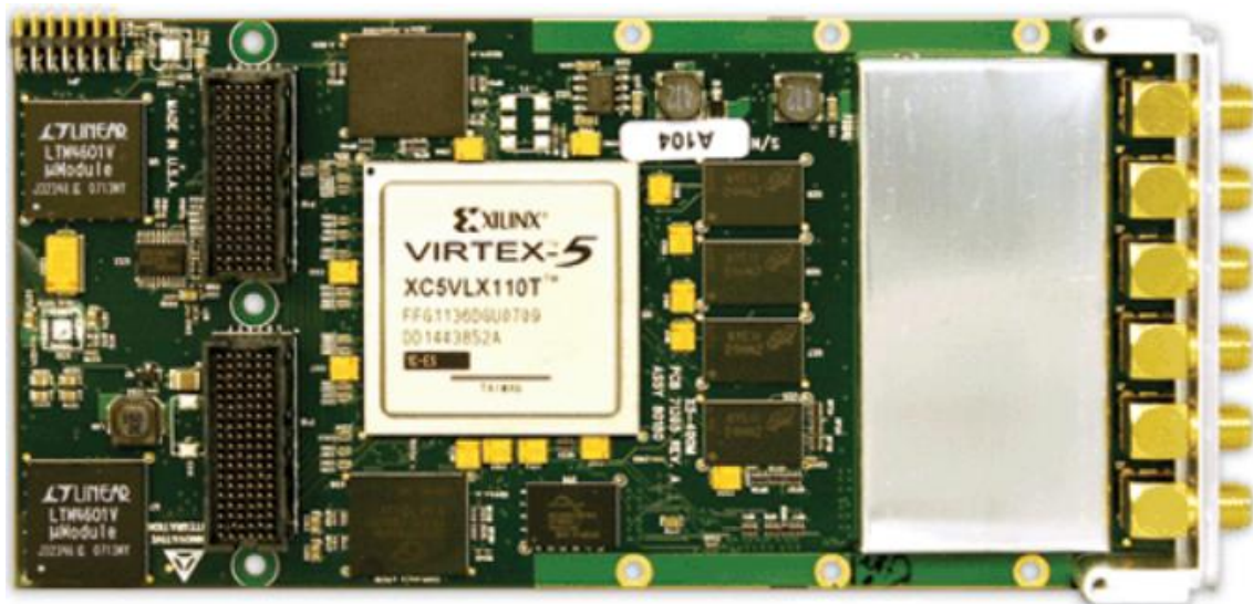
Figure 4-1 The 14-bit ADC used for data acquisition from Innovative Integration (X5-400M)
