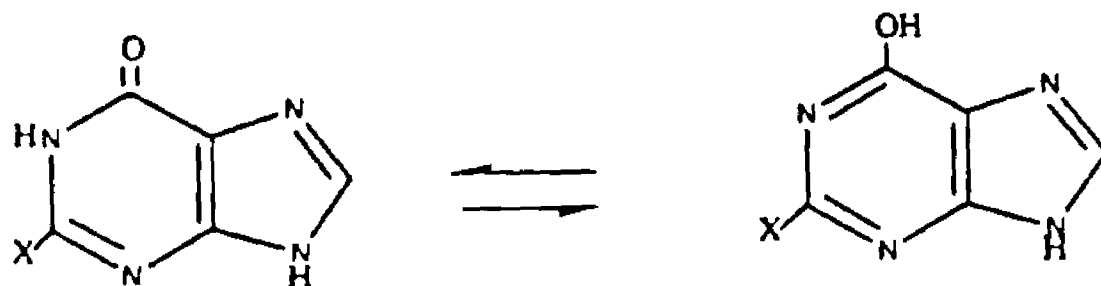
Fig. 2. Lactam-lactim tautomerism of hydroxypurines.
