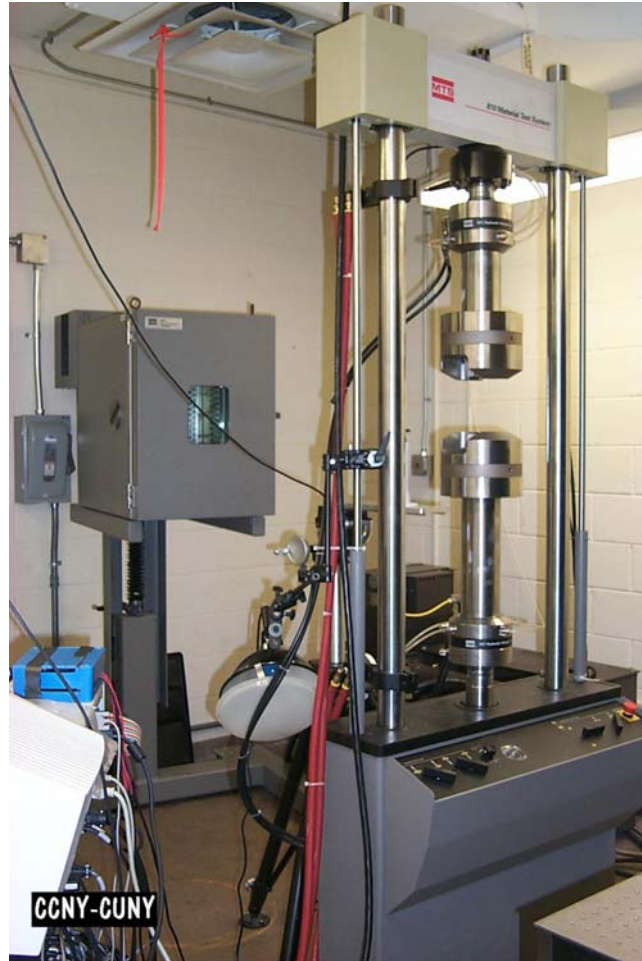
Figure 4-1.2 The MTS universal testing machine equipped with hydraulic grips and an environmental chamber.
