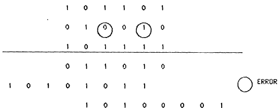
FIGURE 2-2-4c ILLUSTRATION OF A RECEIVED CODEWORD WITH TWO ERRORS
