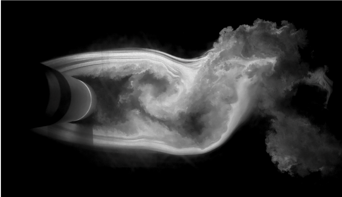
Figure 1: Near wake of cylinder at Re=8 \times 10^4 .
