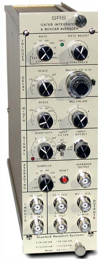
Figure 3.7: SRS 250 - Gated Integrator & Boxcar Averager
