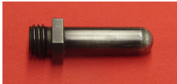
Fig.3.4. A 16-mm hemispherical steel impactor.
