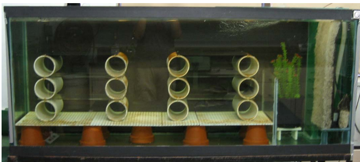
Figure 1.2 – Tank arrangement adopted from Kirschbaum (1987) and Schugardt (1997) for breeding mormyrid fish. Grates along the bottom of the tank allow the eggs to drop down and be separated from fish.
