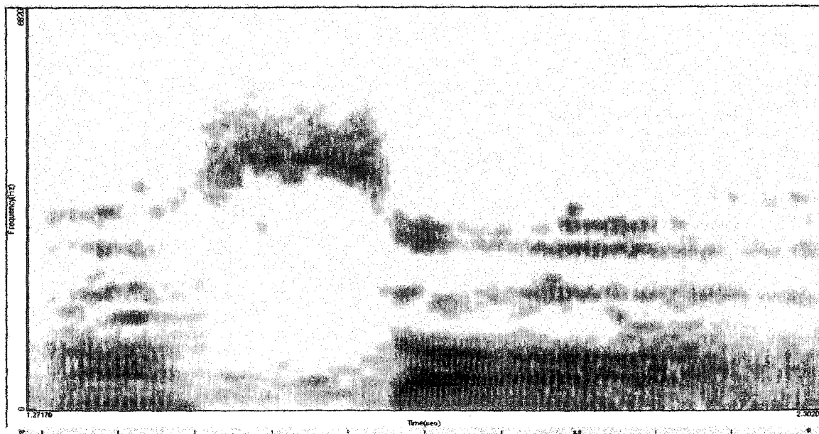
Figure 37. Wideband spectrogram of /asa/ in +10SNR; 16 sine waves (Frequency scale: 0-8820 Hz)
