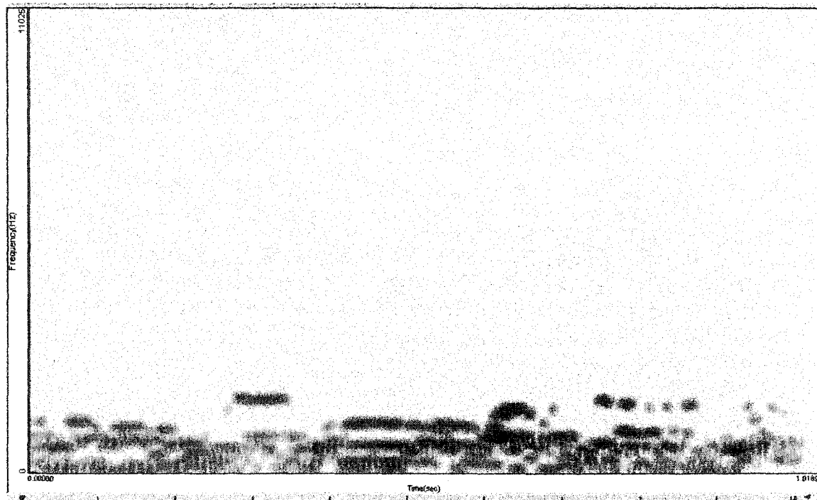
Figure 30. Wideband spectrogram of /aba/ in 0SNR; 4 sine waves (Frequency scale: 0-11025 Hz).
