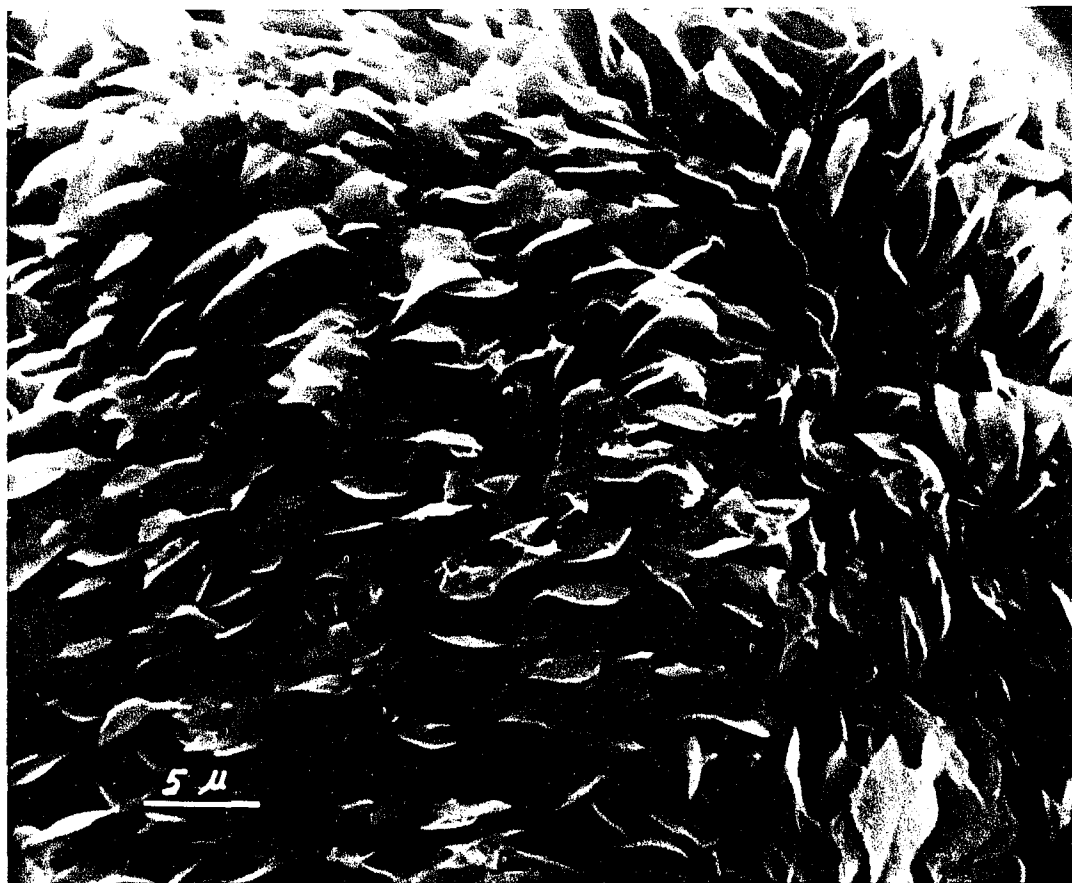
Figure 3.17 Scanning electron micrograph of TPI with \bar{M}_v=2.6 \times 10^5 crystallized from 1% amyl acetate solution at 20°C for two days, treated in suspension with \text{OsO}_4 , viewed from the ends of the ribbons.
