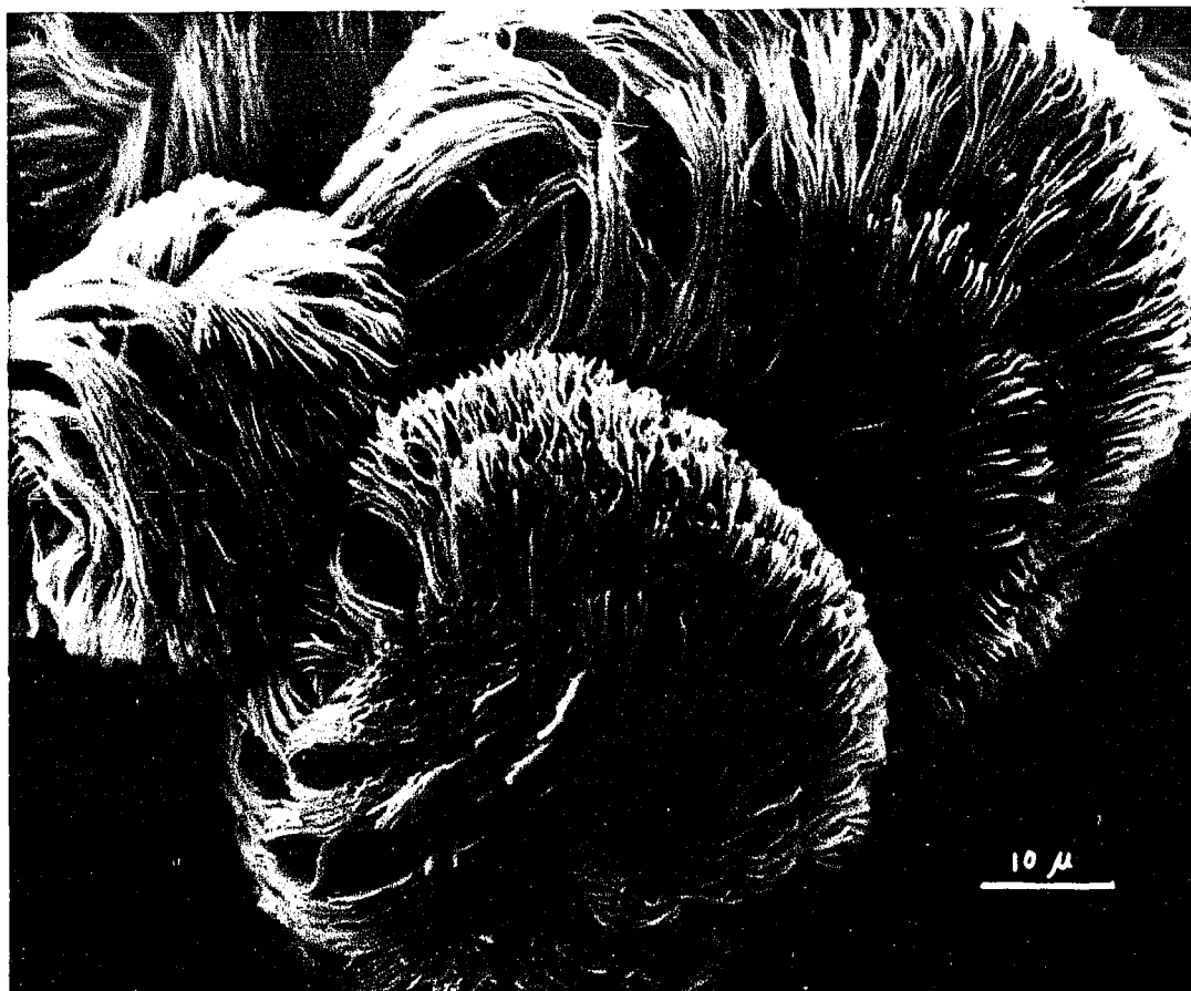
Figure 3.4 Scanning electron micrograph of TPI with \bar{M}_v=1.4 \times 10^5 crystallized from 1% amyl acetate solution at 20°C for 3 hours, treated in suspension with \text{OsO}_4 .
