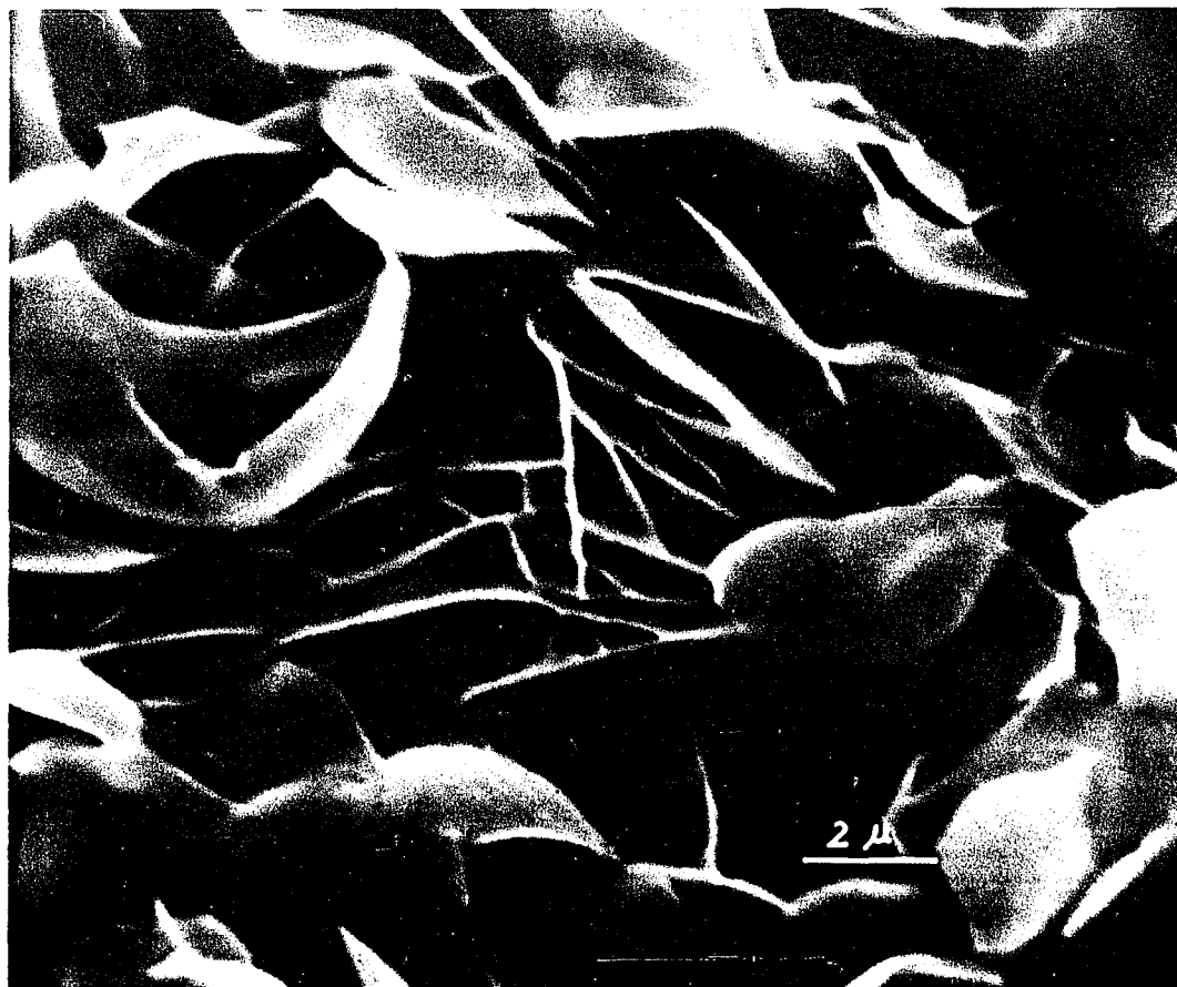
Figure 3.22 Scanning electron micrograph of TPI with \bar{M}_v=5.9 \times 10^5 crystallized from 1% amyl acetate solution at 20°C for 3 hours, treated in suspension with \text{OsO}_4 .
