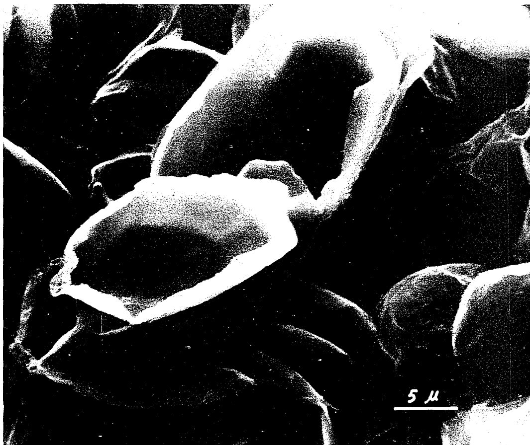
Figure 3.23 Scanning electron micrograph of TPI with \bar{M}_v=5.9 \times 10^5 crystallized from 1% amyl acetate solution at 20°C for 24 hours, treated in suspension with \text{OsO}_4 , minor structures (30-40%).
