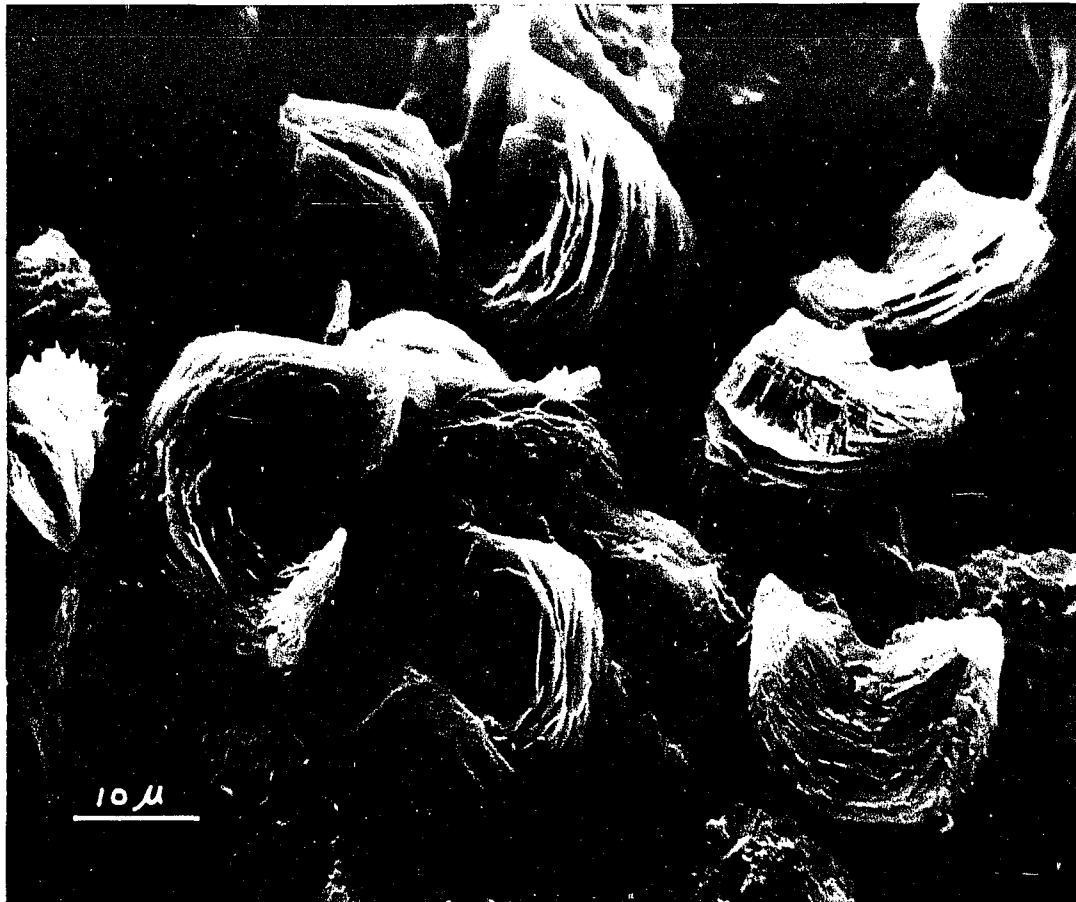
Figure 3.11 Scanning electron micrograph of TPI with \bar{M}_v=1.4 \times 10^5 crystallized from 1% amyl acetate solution at 20°C for 24 hours, ultrasonically vibrated for 3 minutes, treated with \text{OsO}_4 .
