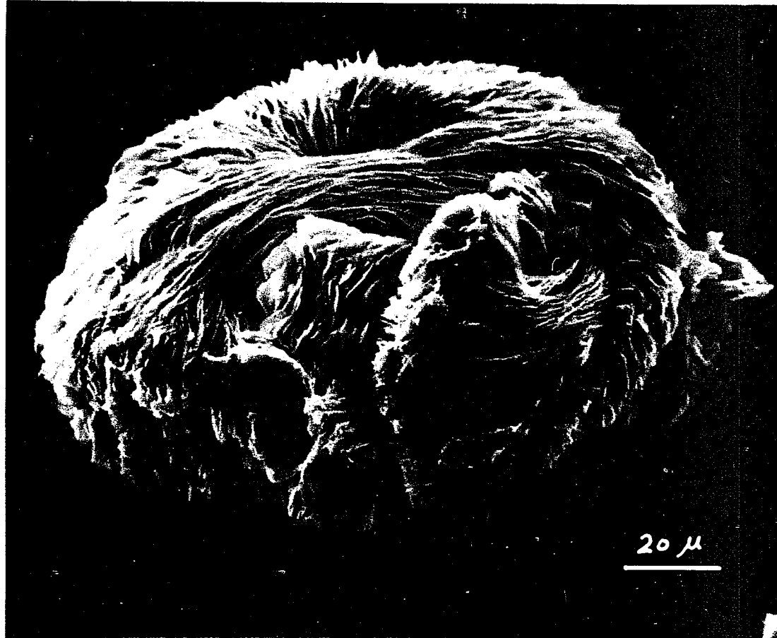
Figure 3.29 Scanning electron micrograph of unfractionated TPI crystallized from 1% amyl acetate solution at 30°C for 4 days, treated in suspension with \text{OsO}_4 .
