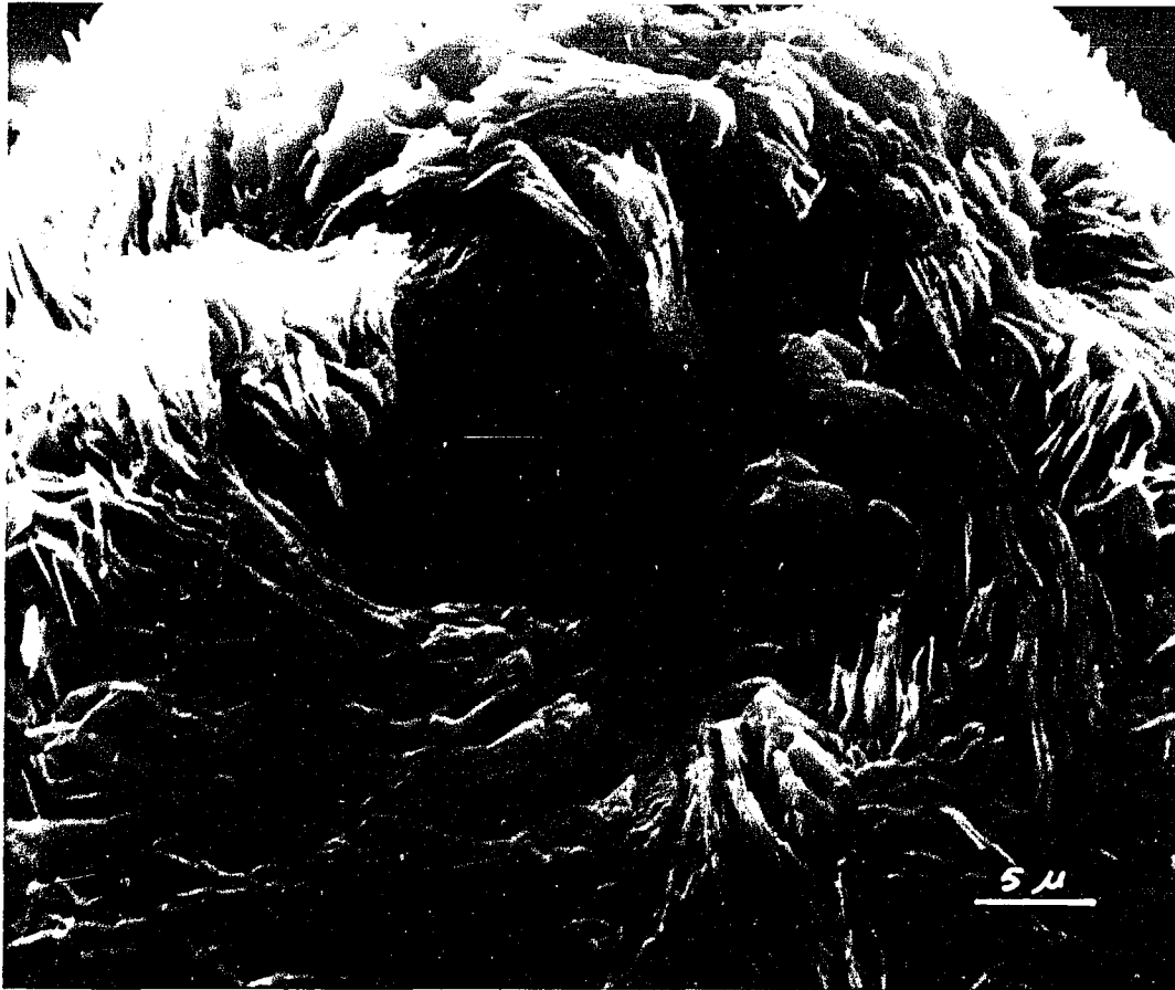
Figure 3.19 Scanning electron micrograph of TPI with \bar{M}_v=2.6 \times 10^5 crystallized from 1% amyl acetate solution at 20°C for 24 hours, ultrasonically vibrated for 3 minutes, treated in suspension with \text{OsO}_4 .
