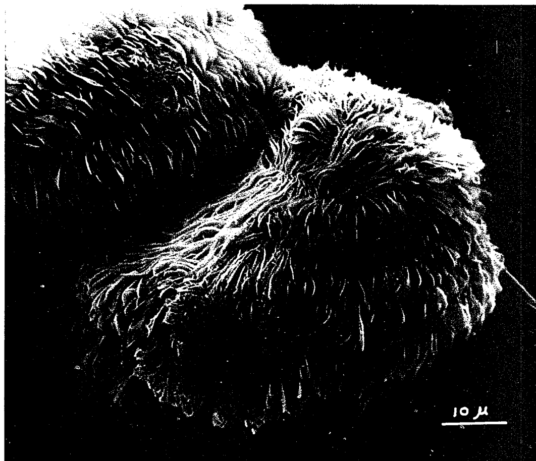
Figure 3.14 Scanning electron micrograph of TPI with \bar{M}_v=2.6 \times 10^5 crystallized from 1% amyl acetate solution at 20°C for 3 hours, treated in suspension with \text{OsO}_4 .
