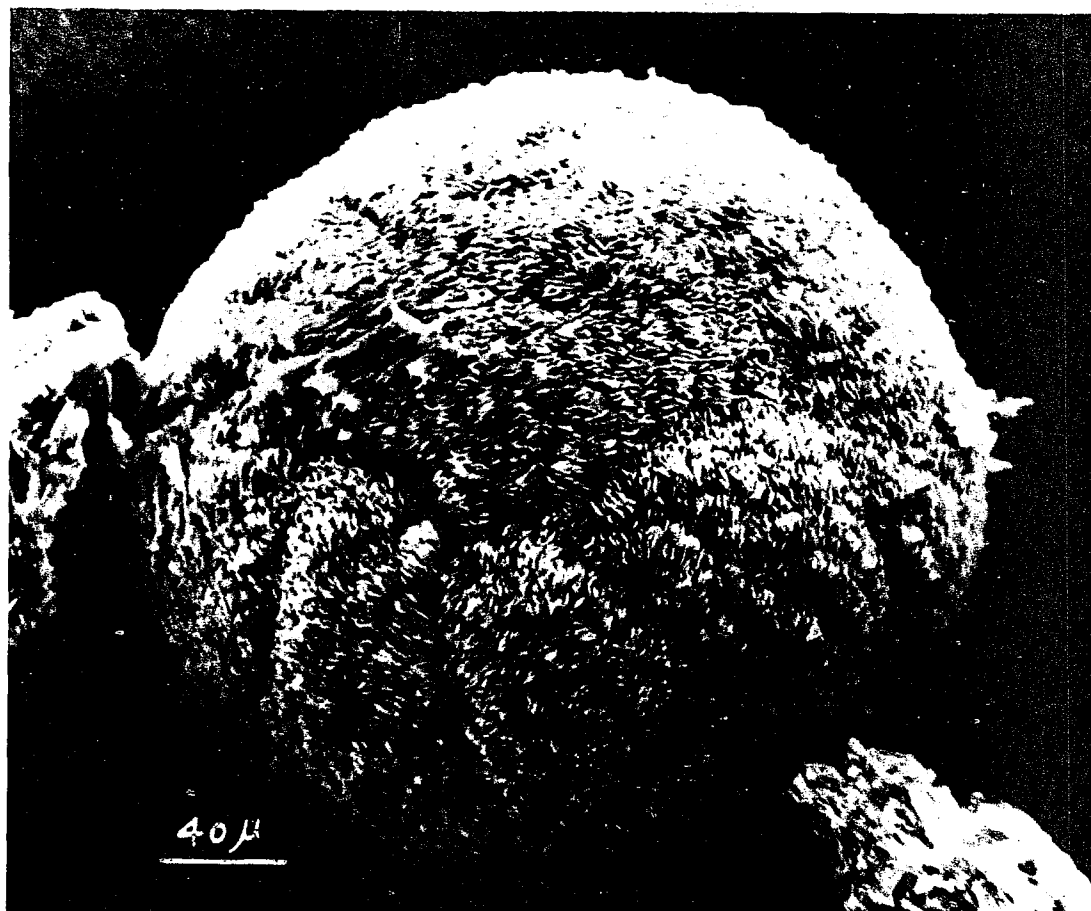
Figure 3.26 Scanning electron micrograph of TPI with \bar{M}_v=2.6 \times 10^5 crystallized from 1% amyl acetate solution at 25°C for 4 days, treated with \text{OsO}_4 .
