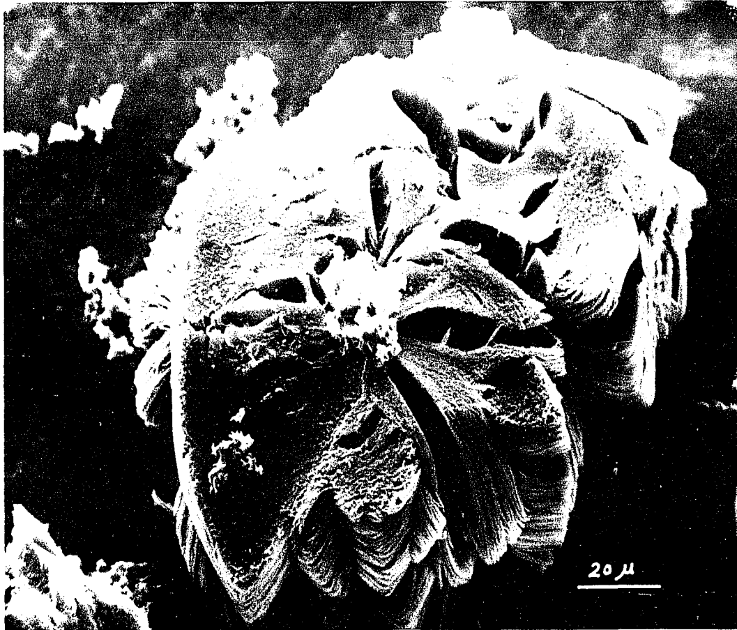
Figure 3.31 Scanning electron micrograph of TPI with \bar{M}_v=2.6 \times 10^5 precooling crystallized ( T_R=31.7^\circ\text{C} ) from 1% amyl acetate solution at 30^\circ\text{C} for 4 days, treated in suspension with \text{OsO}_4 .
