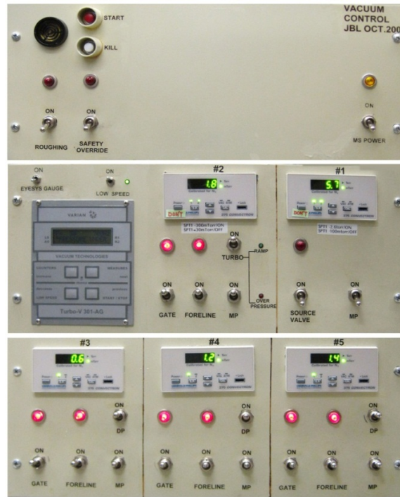
Figure A.1 Front panel of interlock system
