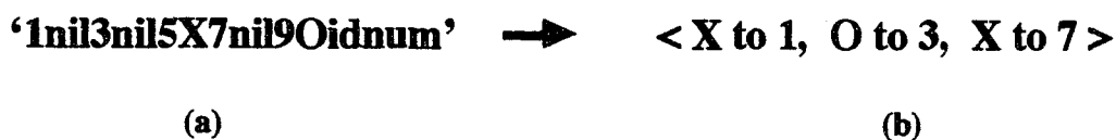
Figure 15: A Context Pair Hash Table entry formed by Update-Hash-Table (a) the key (b) its value
