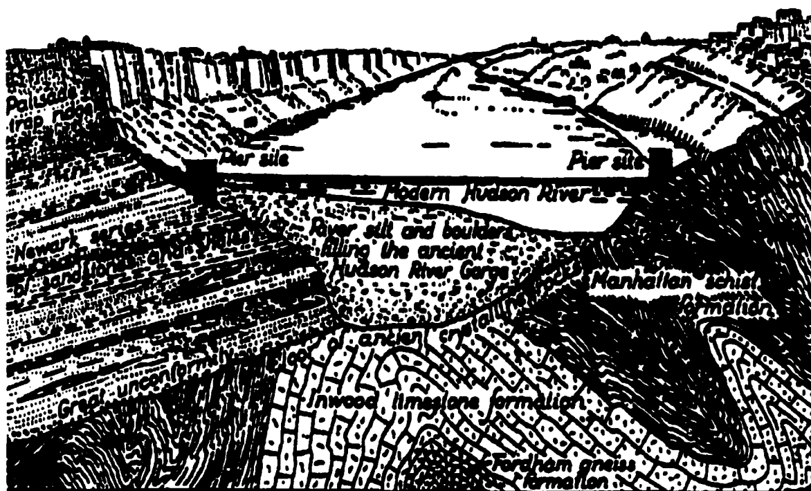
Figure 4. Interpretive geological section across the Hudson River in the vicinity of George Washington Bridge (Sanders and Merguerian, 1997, figure 4, p. 56)
