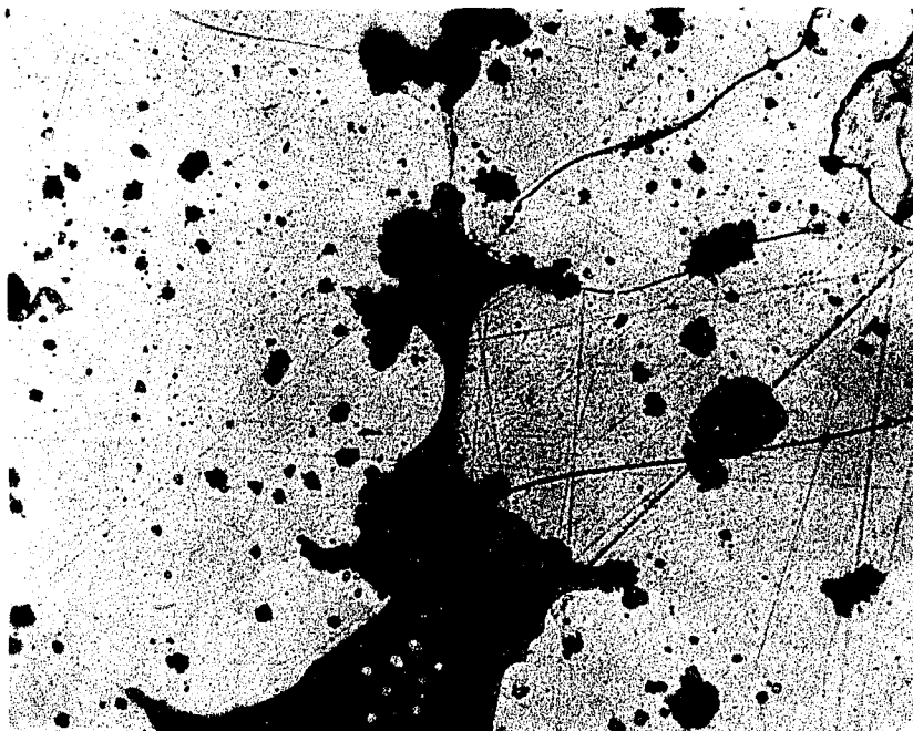
Figure 8. Micrograph of Oxide Formed on \text{TiSi}_2 Oxidized at 800^\circ\text{C} , 320 X.
