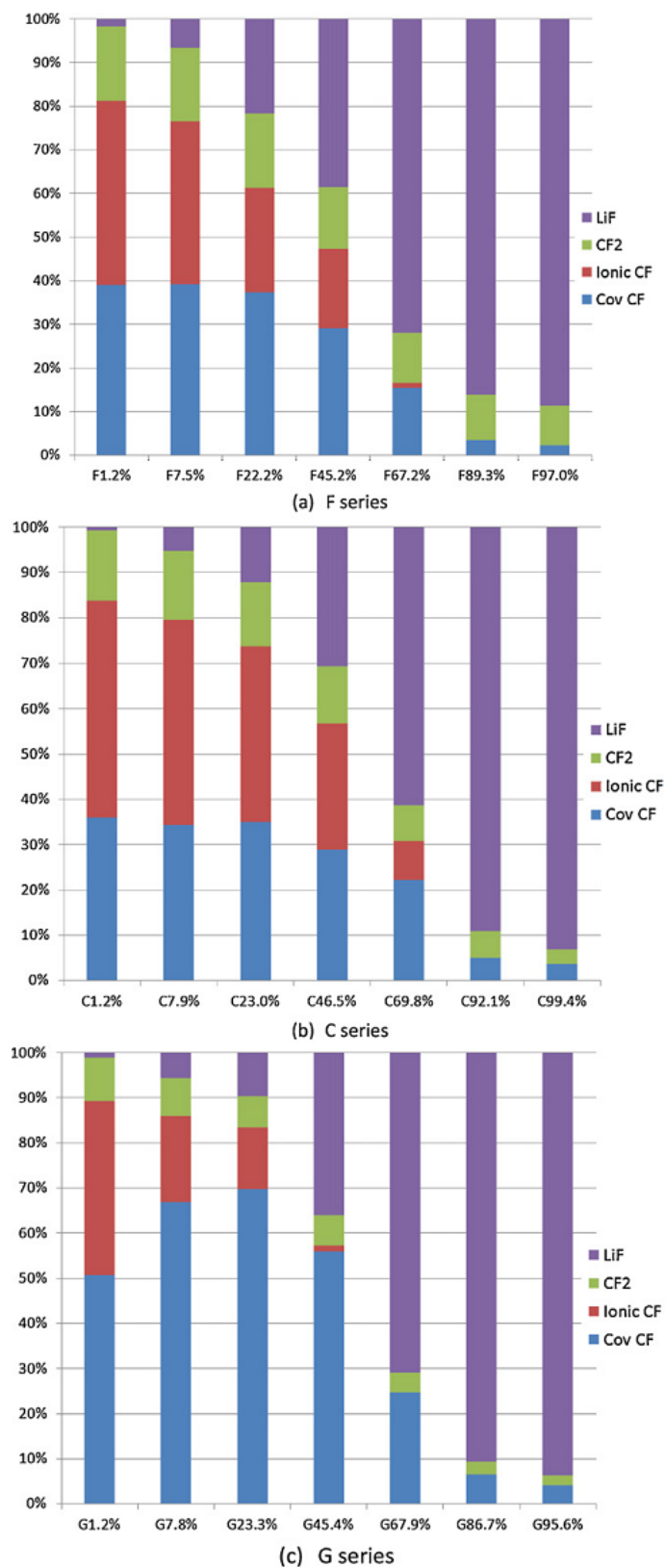
Figure 4.3.7: ^{19}\text{F} MAS NMR deconvolution of Greatbatch discharged F, C and G series.
