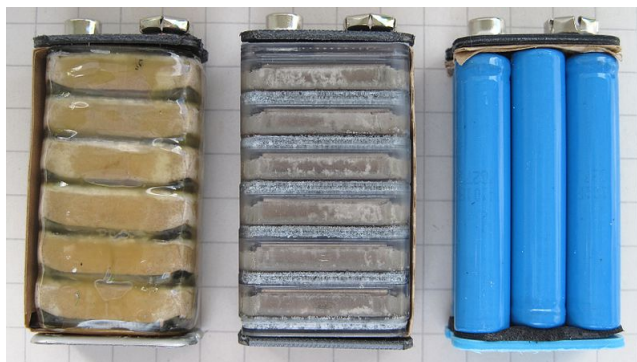
Figure 2.1.1: Three different kinds of 9-volt battery internals.
