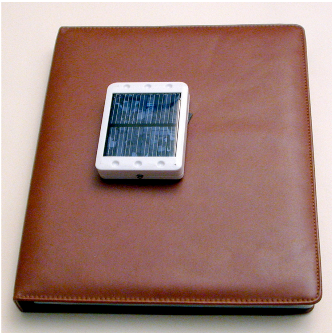
Figure A.8.1. The cover of a talking book, made from a talking photo album and a solar panel to recharge its batteries.
