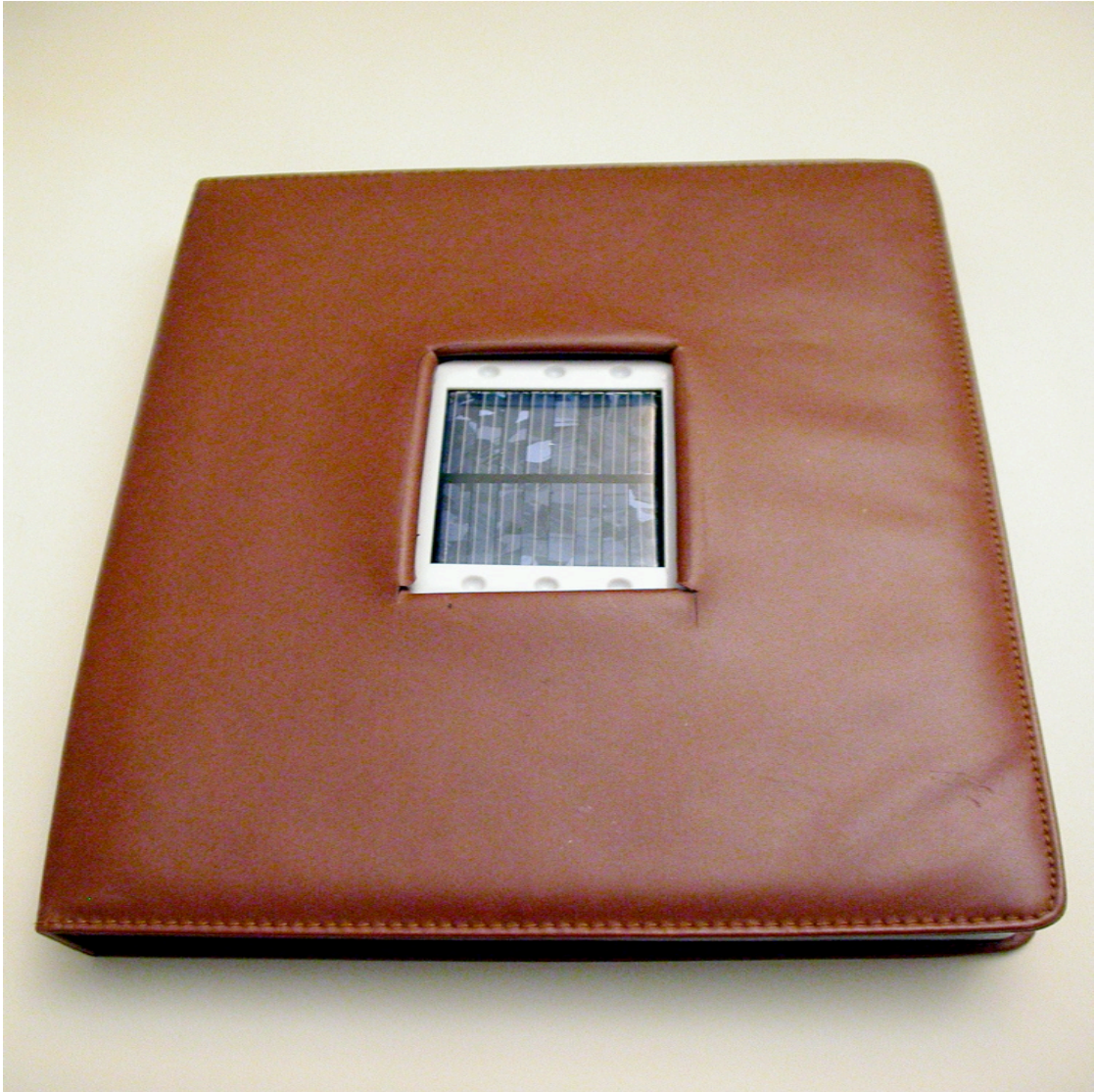
Figure A.8.4 . Solar panel recessed inside electronics compartment, a more durable construction.
