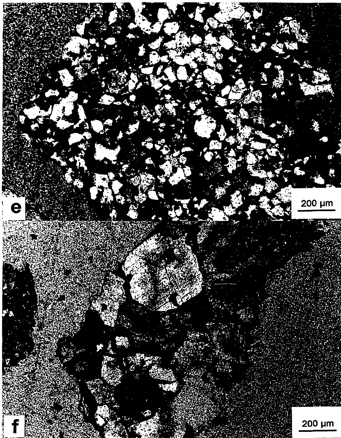
Figure 5-1. (e) Mlf 2-a, upper part of Galway Formation (6460 to 6470 feet). Fine sandstone composed of well-sorted quartz with interstitial pores filled with oil residue. (f) Mlf 2-a, upper part of Galway Formation (6560 to 6570 feet). Crystalline dolostone in which intercrystalline pores contain oil residue. On the basis of the textural relationship between dolomite rhombs and the pore spaces (rhombs projecting into pores; small rhombs "floating" in the pores), these pores are inferred to have formed by dissolution of nonreplaced original calcium-carbonate mud and thus are of secondary origin.
