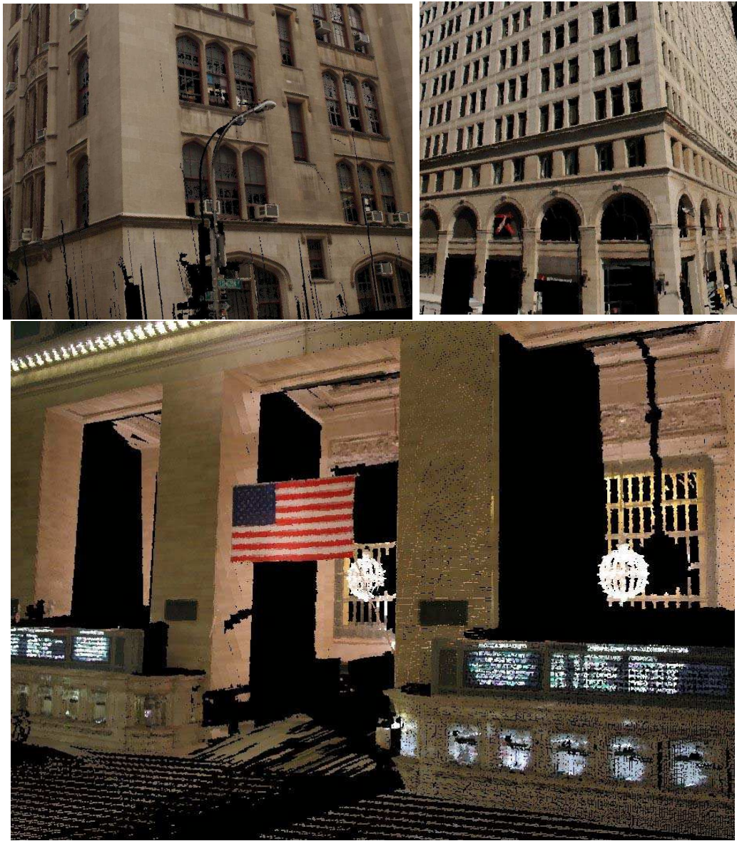
Figure 5.8: Top: Texture mapping details for Building 1 (left) and Building 2 (right). The texture mapped urban structures (windows, street signs, AC units, etc.) show the high accuracy of our registration system. Bottom: Texture mapping details for Building 3. The flag and lights show the accuracy of our registration system.
