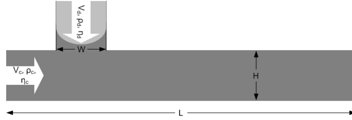
Figure 7.1: 2D Schematic diagram of T-junction. v_d and v_c are the mean velocities of the dispersed and continuous liquid respectively. \eta_d and \eta_c are the dynamic viscosities and \rho_d and \rho_c are the densities.
