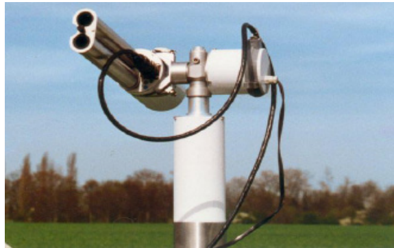
Figure 2.7 The CE 318 automatic sun tracking photometer has been designed and realized to be a very accurate sun photometer with all the qualities of a field instrument.
