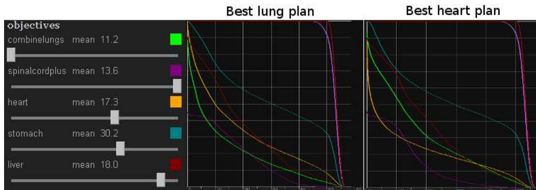
Figure 1.5: IMPT MCO planning system showing the esophagus case. The left panel displays the constraints and the objectives and shows the navigation sliders in positions for the best lung plan. The DVH displays and iso-dose lines are updated in real-time while the user navigates. Here we show the DVHs for the best lung plan and the DVHs for the best heart plan, which together display the range of planning options regarding these two critical structures. (Patient data courtesy of Dr. T. Hong.)
