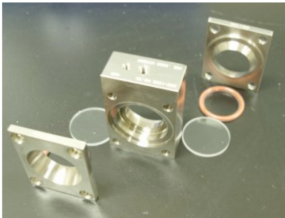
Figure 3.4: Demountable SANS cell used for to hold sample for SANS analysis. (reference: http://www.ncnr.nist.gov/programs/sans/equipment/dem_cell.html )
