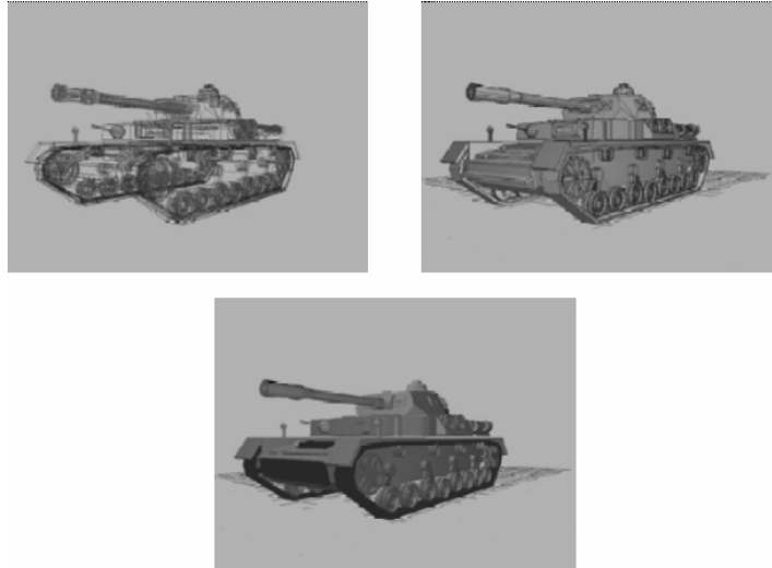
Figure 5.41: Synthetic images of the targeted object: a wireframe model (top, left), a principal model (top, right), and a textured 3-D model (bottom)
