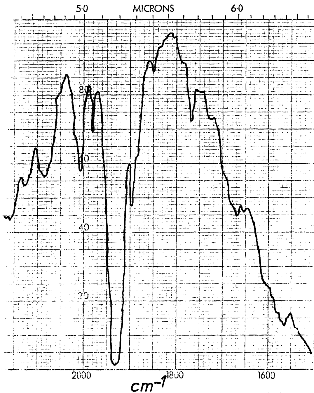
Figure 9. Infrared spectrum of W(^{13}CO)_6 dissolved in n-hexane. Spectrum illustrates the 90% enrichment of labeled complex.
