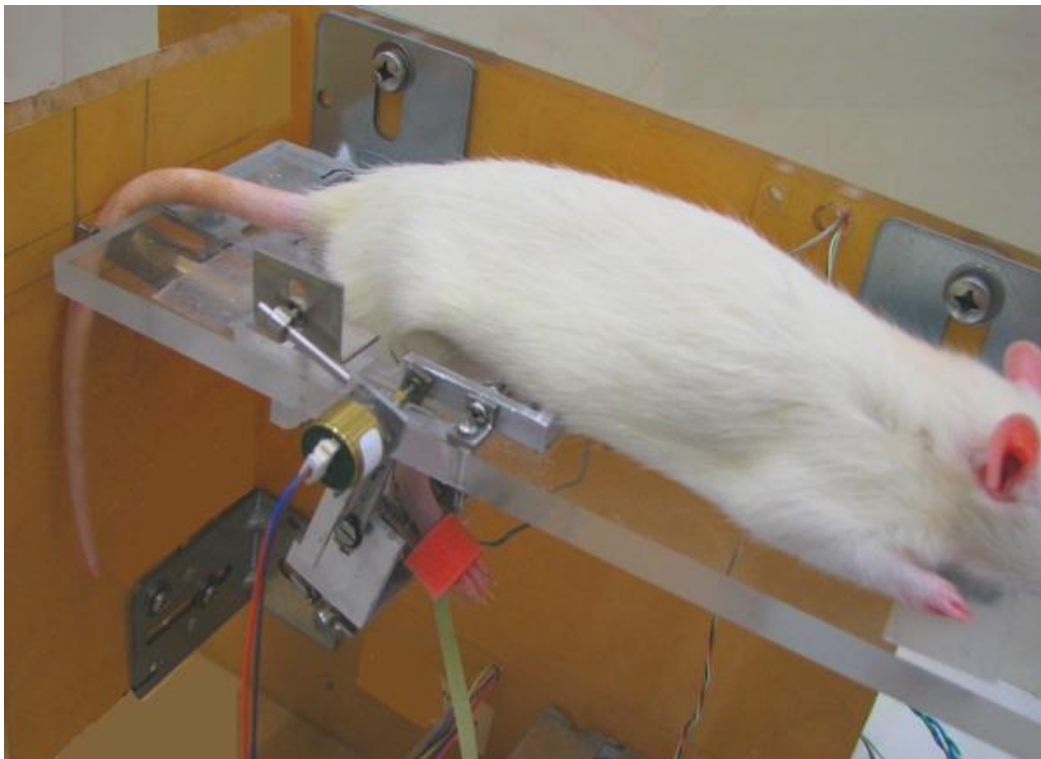
Figure 2.2 (Upper) Schematic diagram of the JMLS design and (Below) Photograph of the experimental setup with an animal undertaking motion and loading experiment.
