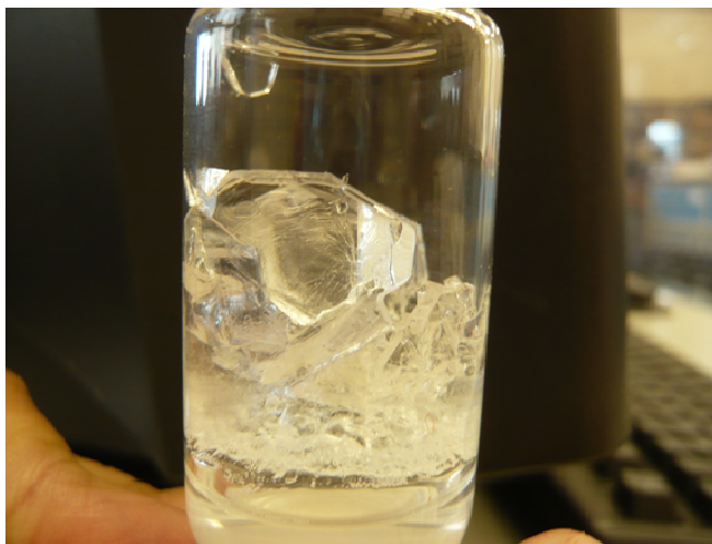
Figure 9.7. Large hydrate crystal formed under magnetic field.
