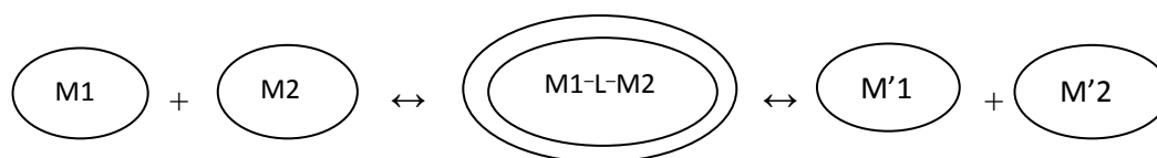
Figure 14. Scheme for inner-sphere mechanism of electron transfer.
