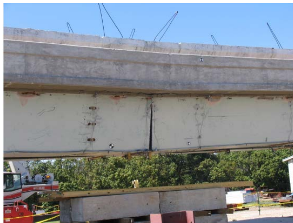
Figure 5.14 - Fracture view with the bin loaded on the top [Neuman, 2009]
