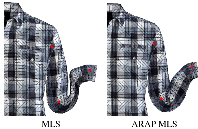
Figure 7.4: Comparison of MLS and ARAP MLS deformation results. Notice that the MLS version induces excessive distortion in the sleeves. This result can be improved, however, by using exterior control points (see Sec. 7.3.5).
