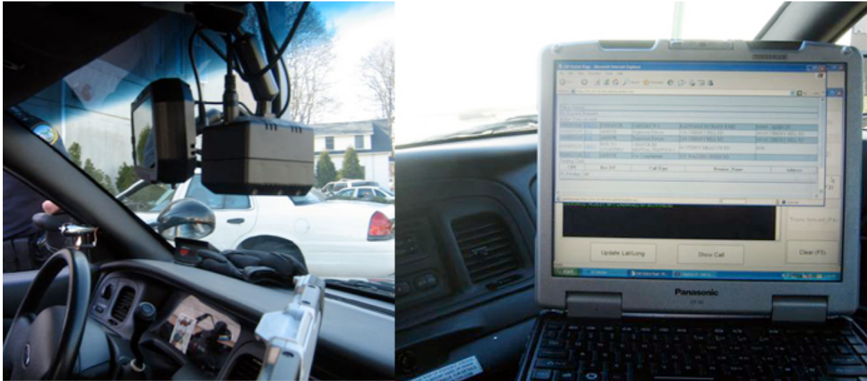
Illustration 13: Inside the Belleville patrol cars, detail of dash cam mounted on rearview mirror (left) and the LEAS computer terminal (right)
